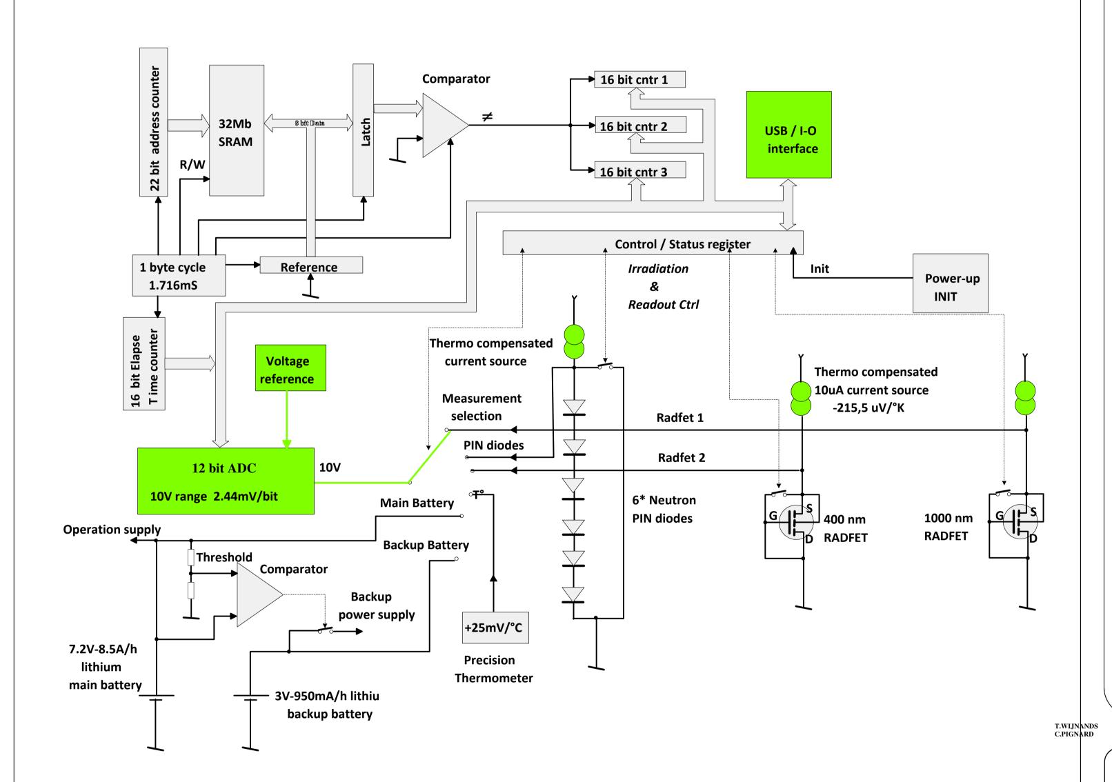
Components in green are not exposed to radiation and are located in the remote readout unit. Connectivity to a PC is via the USB interface.
