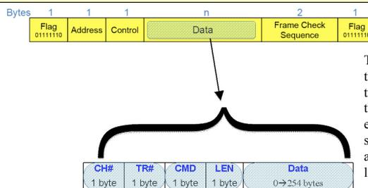
The channel number (CH#) identifies the user port to be addressed, the transaction identifier (TR#) facilitates the verification of the command execution, the command type (CMD) specifies the read or write operation, and the length (LEN) specifies the length of the Data field.
