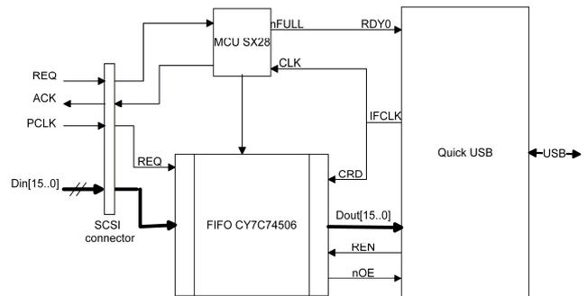
Figure 1: The block diagram of the Parallel to Serial Flow Converter (PSFC).
