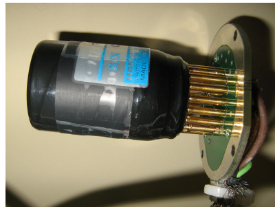
Figure 2: the R5505 PMT mounted on the CASTOR base
