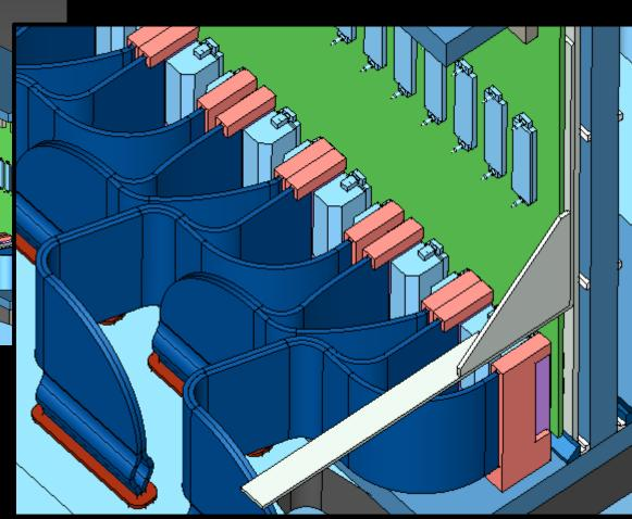
Testing connections during the pigtail installation sequence would involve installing and then removing DCBs; they obstruct pigtail installations in general
