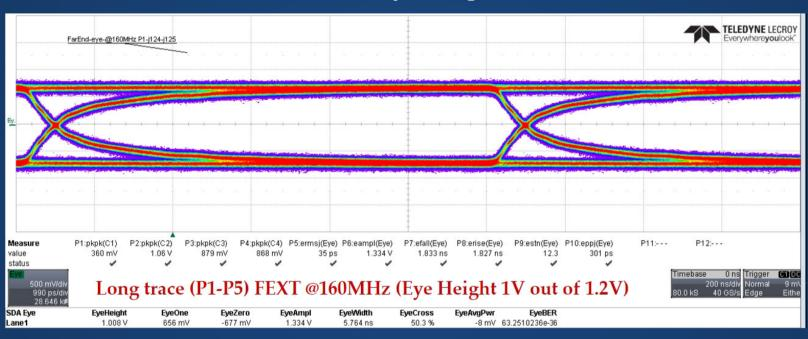
Eye wide open @160MHz, S/N>10 and jitter(RMS) around 36ps (12ps due to the setup)
