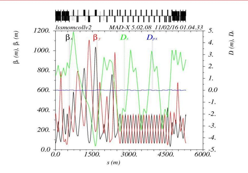
Improved versions based on fodo canal have been developed: aim is to improve the dispersion management by different ways: fodo cells phase advance change and dispersion suppressor quads strength matching.
