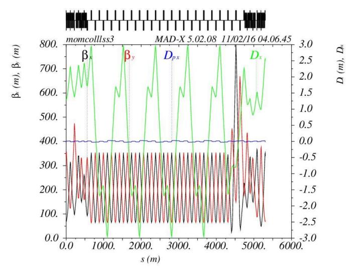
Fodo cells phase advance has been reduced from 90° to 60° withtout any other change. Dispersion at location of primary collimator is 5.1m.
