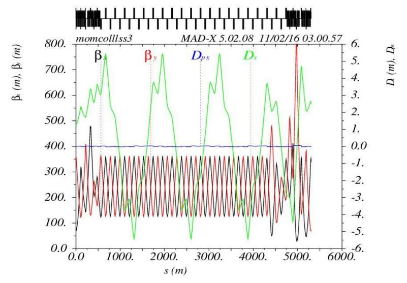
Fodo cells phase advance has been reduced from 90° to 60° with additional quads matching to improve dispersion.
