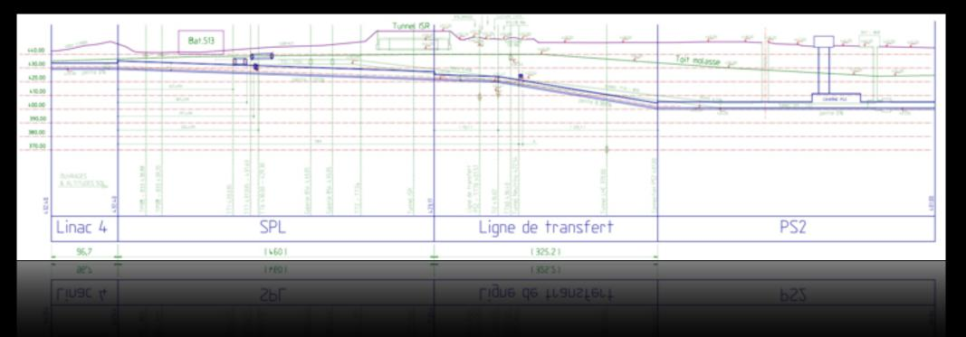
The SPL tunnel trajectory keeps necessary distances from existing tunnels/buildings (computing building 513, nTOF, transfer lines...)
