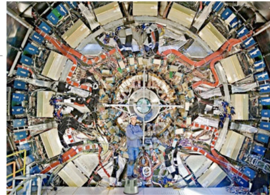
Fig. 1. The ATLAS SCT (semiconductor tracker) detector. The thick red cables on show feed the detector with half of its power - adding more will take up even more space. Click to enlarge image
