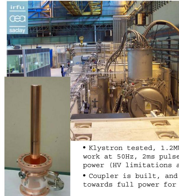
• CryHoLab (horizontal cryostat) has cavity installed.
