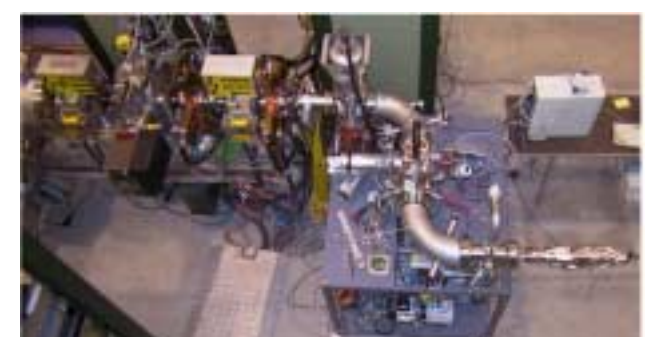
ASACUSA : Interaction region with ESA (ElectroStatic Analyser)
