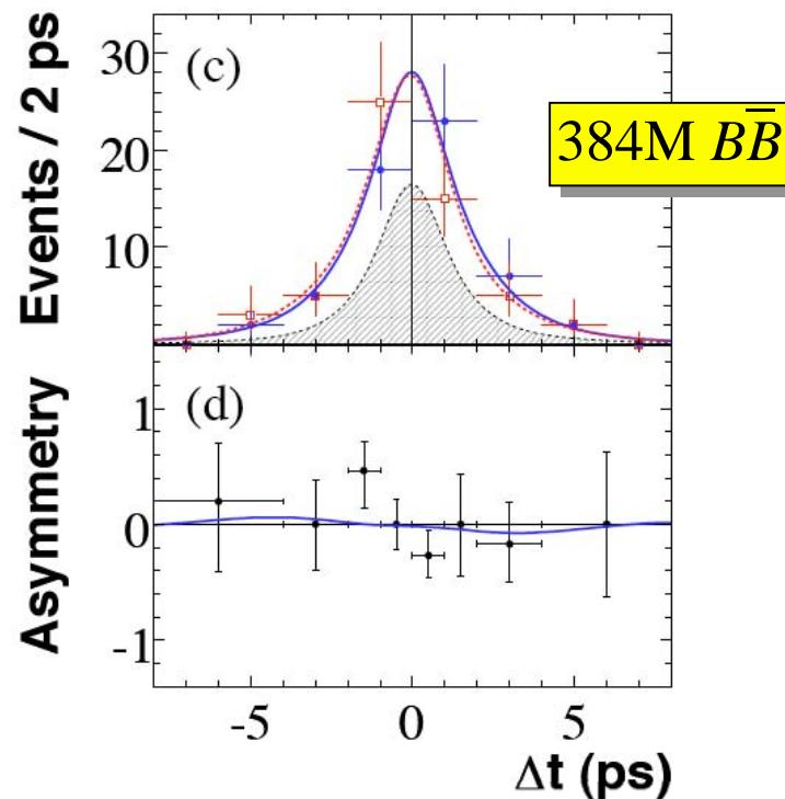
$$\begin{aligned}\text{"sin}2\beta\text{"} &= +0.58 \pm 0.10(\text{stat}) \pm 0.03(\text{syst}) \\ \mathcal{A} &= -0.16 \pm 0.07(\text{stat}) \pm 0.03(\text{syst})\end{aligned}$$
