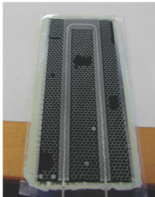
Missing honeycomb glue locations
