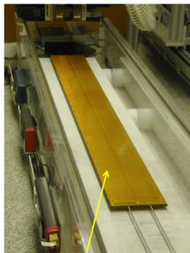
Kapton power/signal cable cured into carbon fiber facing
