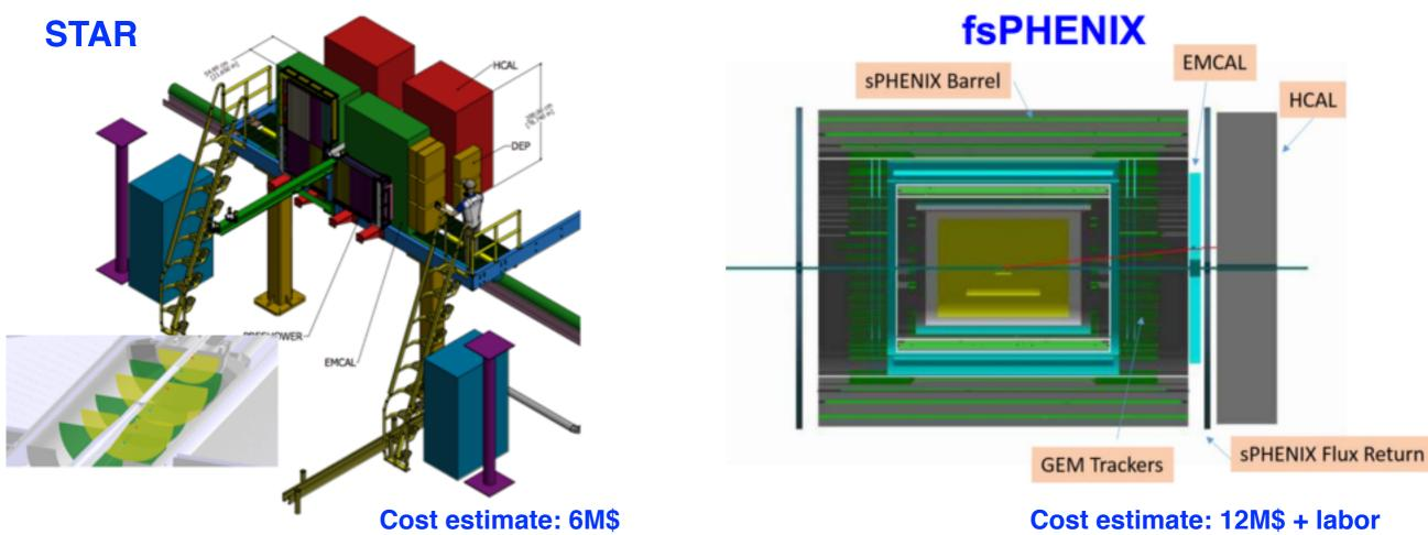
Requires a combination of electromagnetic and (new) hadronic calorimetry, and tracking.
