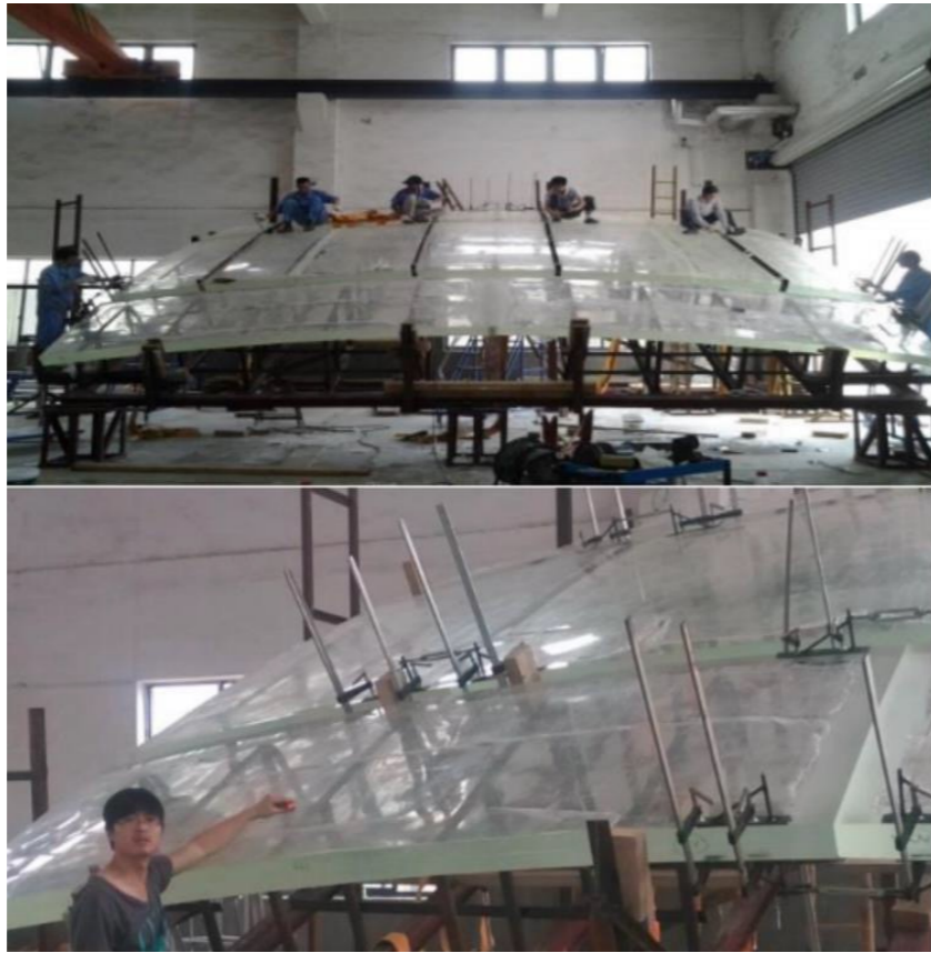
Forming panel size: 3 m x 8 m x 120 mm
