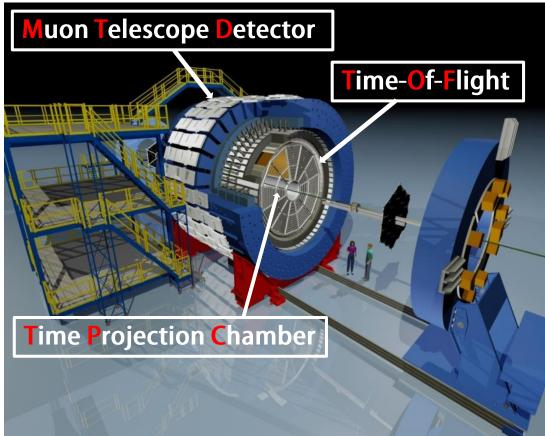
Muon identification: based on energy loss measured by TPC and the position/time differences between MTD measurements and TPC track projection.
