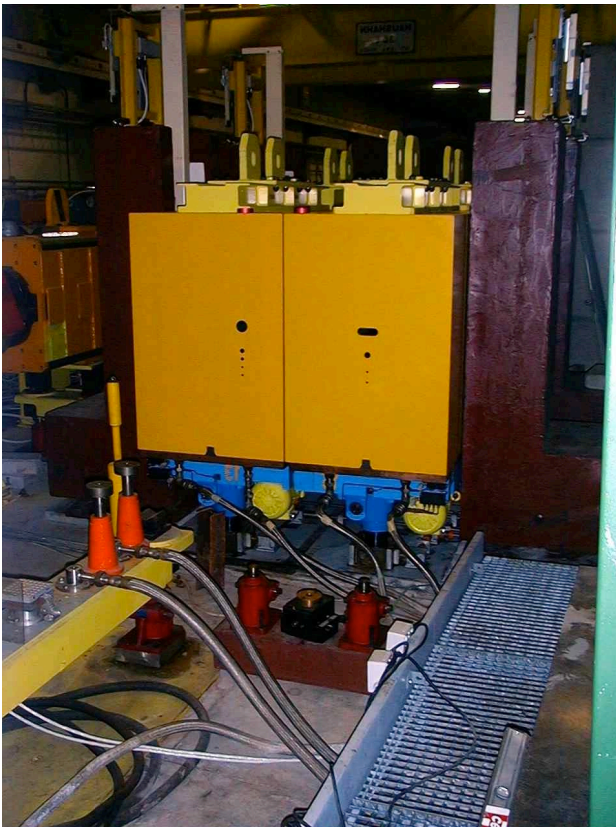
Figure 1: A TAX assembly in TCC2 (H2/H4 beams) - before the outside shielding is put in place
