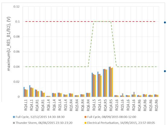
New threshold of 40 mV already implemented for 10 MQY magnets. Not possible for 2 MQY magnets
