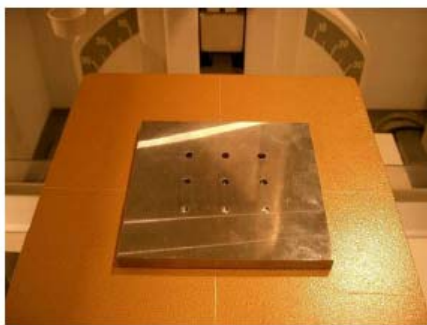
Iron plate with 10mm thickness Hole diameter : 6mm
