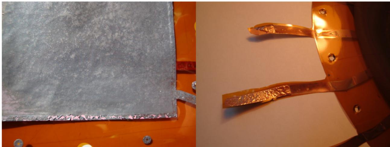
Apart from oxidation, deposits of a polymer are found on the electrodes. Will try heat cycle in moderate vacuum. GEMS may end up clean enough for a sealed detector.
