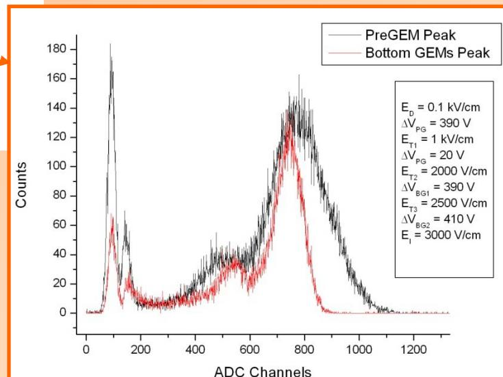
We managed to find a configuration in which the parameter  $G_{\text{PreAmpGEM}} * \epsilon_{\text{GateGEM}}$  is very close to 1. In this case we observed an overlapping of the two main peaks obtained through the conversion in the drift gap and below the Gating GEM. The spectrum for the Bottom GEMs was acquired with closed gate ( $\Delta V_{\text{GateGEM}} = -20 \text{ V}$ )
