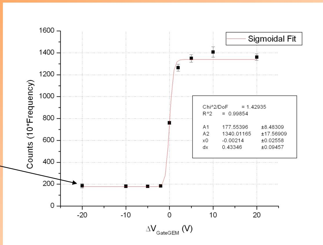
Varying the voltage on the Gating GEM by 40 V, it is possible to completely close the gate. The obtained counts are higher than zero @  $\Delta V_{\text{GateGEM}} = -20$  because of the conversions after the gate.
