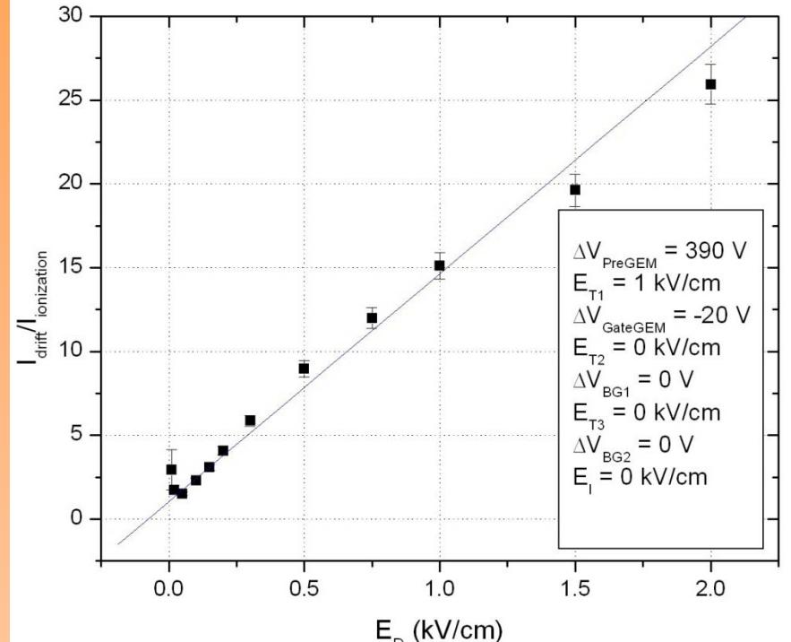
Using a Drift Field of 0.1 kV/cm (the same that is usually present in a TPC gas volume), the NIF @  $\Delta V_{\text{PreAmpGEM}} = 390 \text{ V}$  is 2-3.
