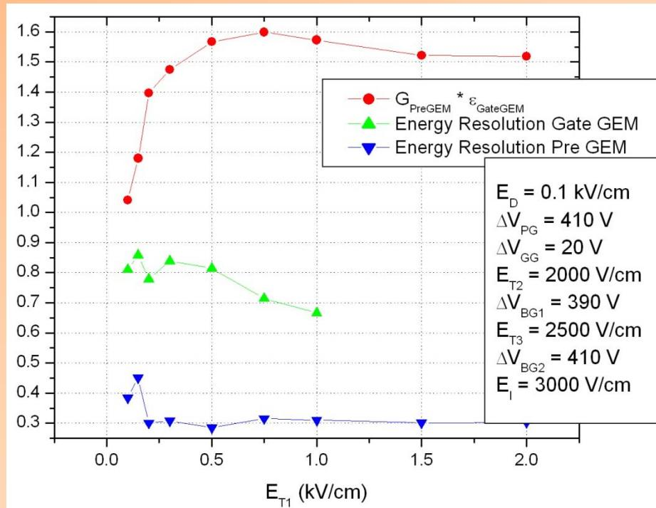
Increasing  $E_{T1}$  value has two opposite effects: the extraction efficiency of the PreAmpGEM is higher but the loss of the electrons on the top of the Gating GEM is increased. We managed to find an optimum between these two behaviours
