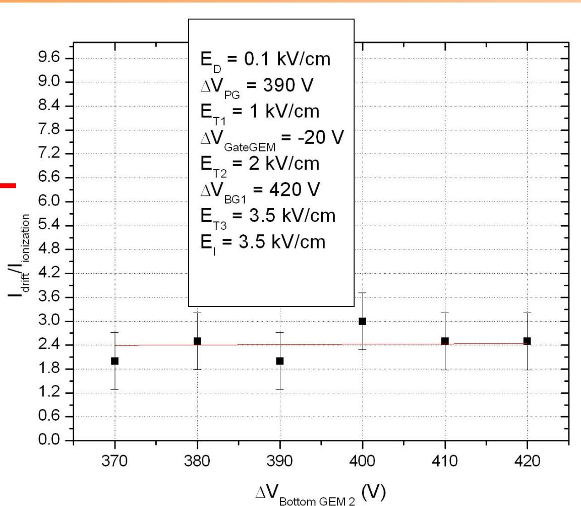
With open gate ( $\Delta V_{\text{GateGEM}} = 20$ ) the point at 400 corresponds to an effective detector gain of about 3000
