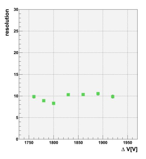
Energy resolution of Resistive-Thick-GEM at several  $\Delta V_{GEM}$
