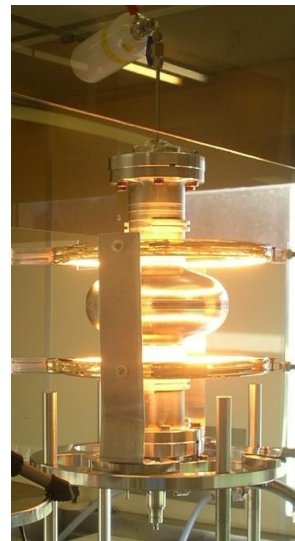
800° C annealing and 120° C baking
