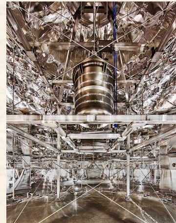
Cherenkov Detector Tank instrumented with 84 high-QE 8" PMTs Active rejection through coincidence tagging*
