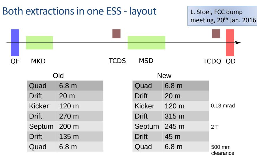
We wanted to shift the TCDS (and thus the septum) as far downstream as possible, to gain more bunch separation through a bigger lever arm.
