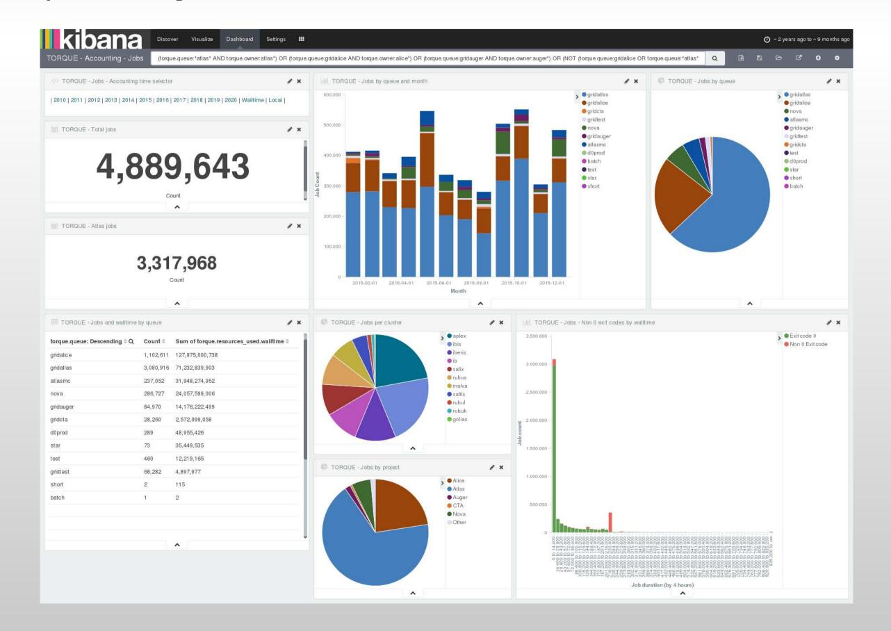
Elastic Stack is used to process all relevant log files. The figure shows an example with accounting graphs and figures from Torque log files.
