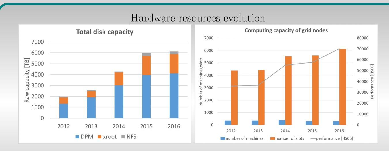
Resources are almost annually upgraded using budget of projects. All subclusters connected to the EGI grid are based on x86\_64 technology, using the same OS (SL6), and jobs are distributed from single Torque server.
