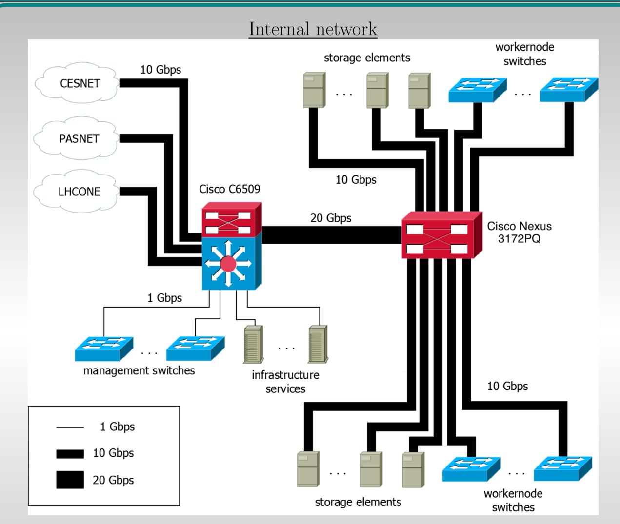
All disk servers are connected via 10 Gbps to the central CISCO Nexus 3172PQ switch. Worker node connection is 1 Gbps to local node switches which have 10 Gbps connection to the central switch. Clusters for parallel computing have independent internal network with outside connection just 1 Gbps. Parallel jobs use QDR Infiniband (not shown).
