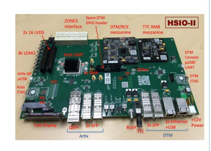
All functionality required in HSIO for the integration with the ATLAS TDAQ is contained in a single Artix FPGA:
