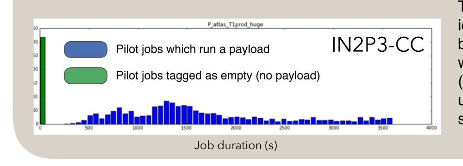
This plot shows the clean identification of empty pilots (green) by combining site batch records with PanDA JobArchive records (method 2). This result validates the use of CPUtime threshold for other sites (method 3).
