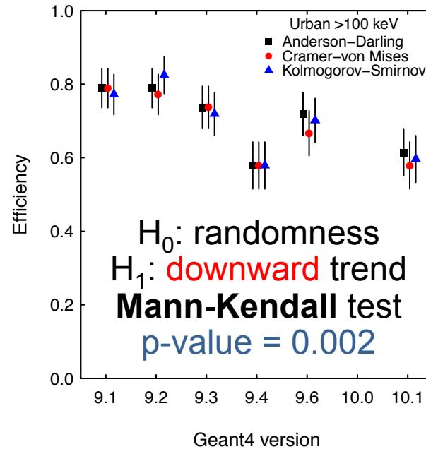
Trend of compatibility with experiment as a function of Geant4 version for different physics configurations
