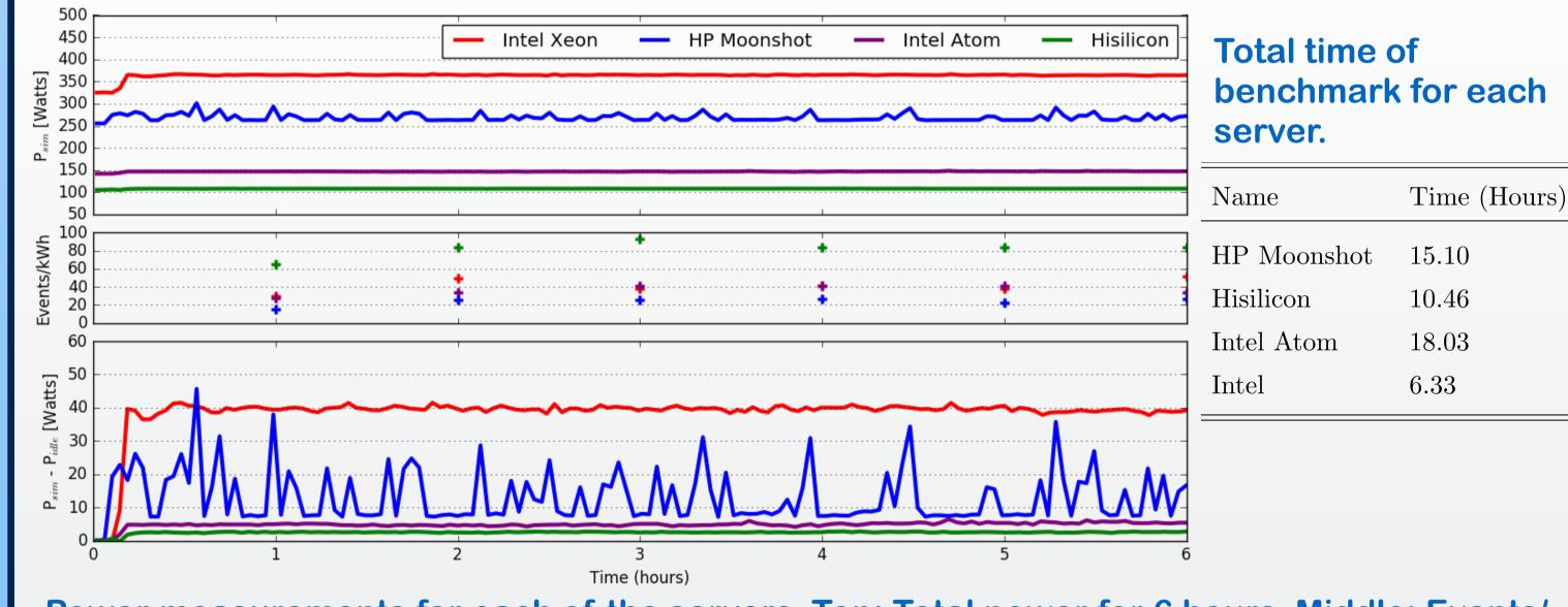
Power measurements for each of the servers. Top: Total power for 6 hours. Middle: Events/ kWh calculated for each hour. Bottom: Idling power of each server subtracted from total power when running simulation.
