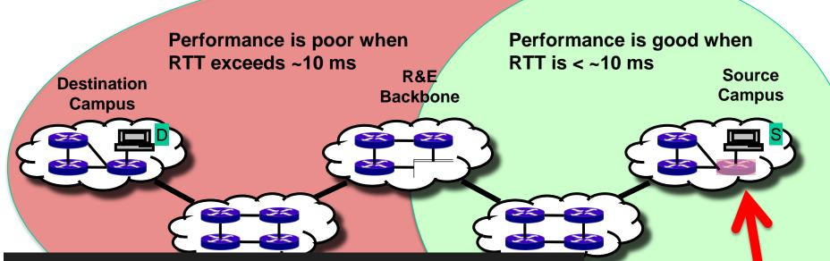
0.0046% loss (1 out of 22k packets) on 10G link
