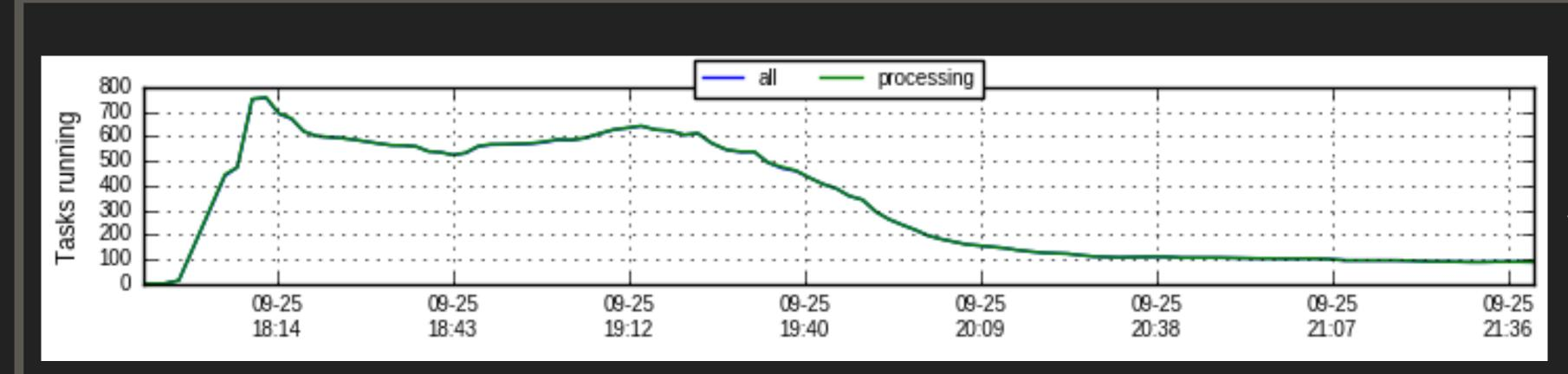
**PROBLEM:** Processing runs have tails. Consider a project with N workflows, where W<sub>N</sub> depends on  $W_{N-1}$ . For N \* (tail length) time, processing is running far below capacity!
