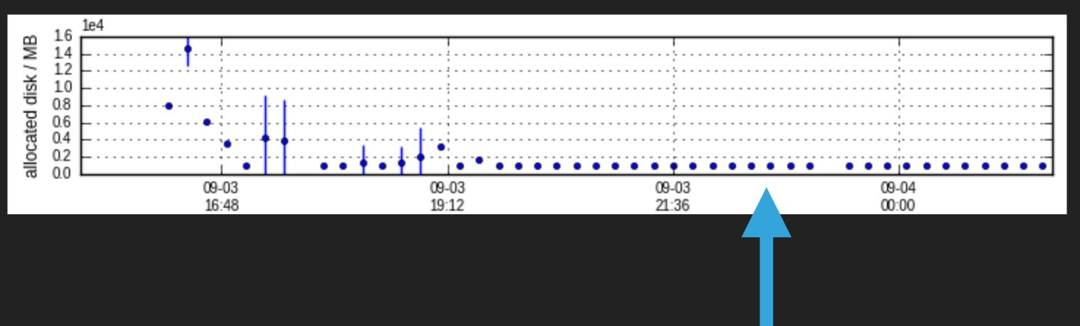
WQ isn't sure how much disk the task needs, so it starts out by taking up the whole worker. As tasks return, the disk allocated settles to the real requirement.
