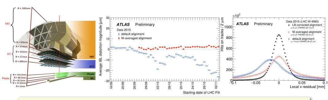
An example: The Insertable B-Layer (IBL) exhibits temperature-driven distortion
