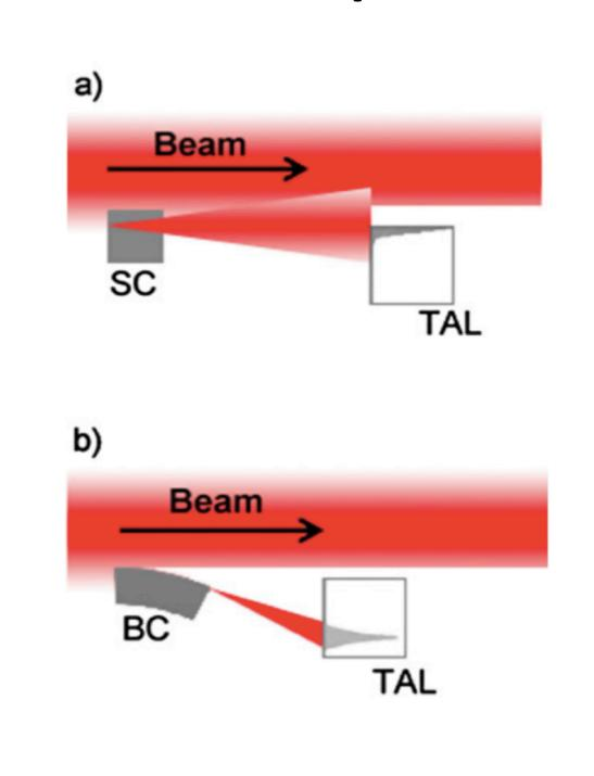
In a hadron collider a multi-stage collimation system is used to absorb the beam halo particles preventing quenches of its superconducting magnets and reducing the collider experiment background. A crystal can be used as a primary collimator to deflect particles of the halo toward a secondary collimator. The main advantages of this scheme are the possibility to deflect the beam out and reduce the beam losses.
