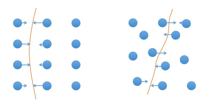
In such case the Coulomb potentials of single atoms can be replaced by an average continuous potential of the plane (string) and the particle dynamics can be described by the interaction with the atomic plane (string) as a whole.
