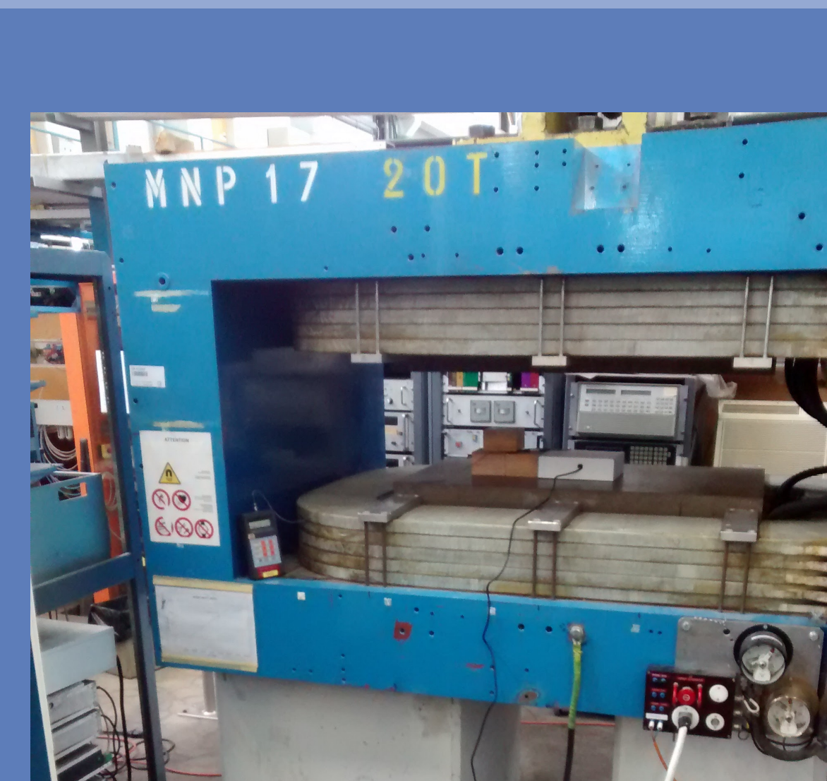
DCES electronics during magnetic field torture test
