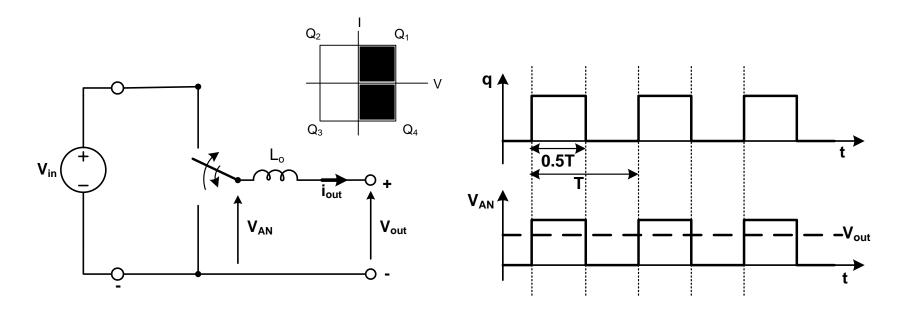
$V_{out} = D.V_{in} \qquad 0 < D < 1$
