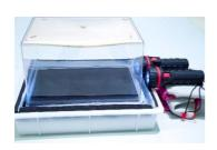
At first, you will only see a rain-like mist of alcohol. Place your torch lights in a way, that they illuminate the alcohol mist right above the metal plate – that is the sensitive area of the chamber.
