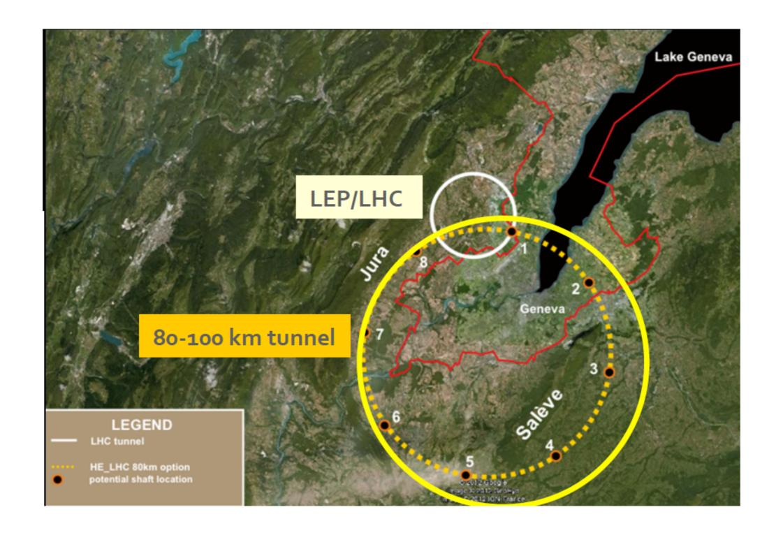
A possible implementation of the 80 km tunnel (dashed) that would host FCC-ee and FCC-hh. 100 km version under study
