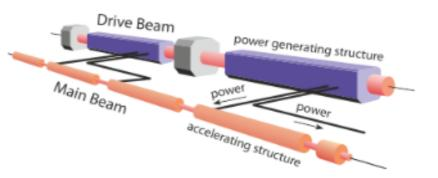
This drive beam is decelerated in special Power Extraction and Transfer Structures (PETS), and the generated RF power is transferred to the main beam. This leads to a very simple tunnel layout without any active RF components (i.e. klystrons).
