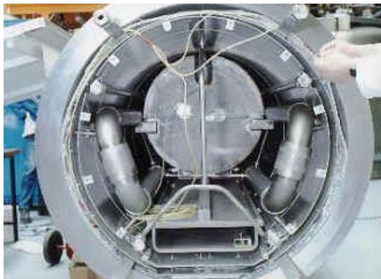
view of the horizontal cryostat opened with a LHC bus bar measurements
