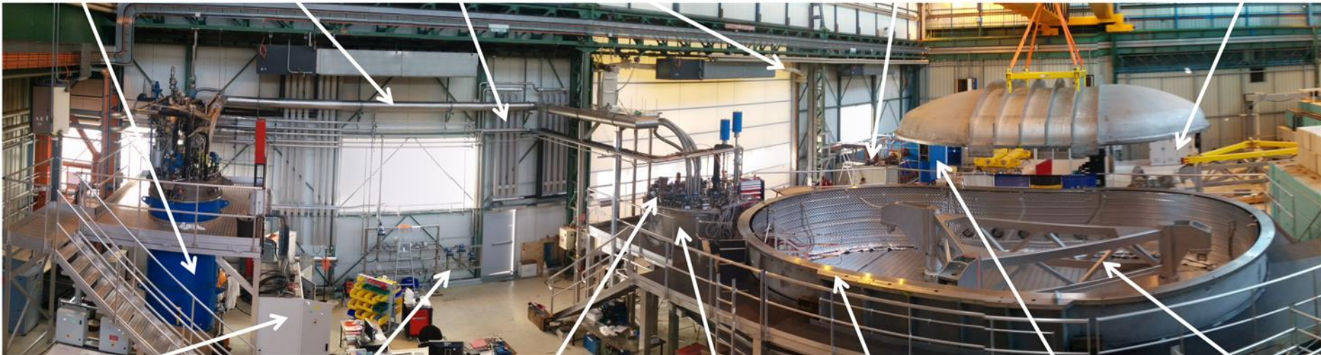
Process and control cabinets Warm valves HTS current lead Valve box Cryostat Power supply Test frame
