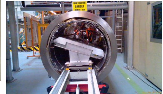
R 3 B-Glad coil prototype
