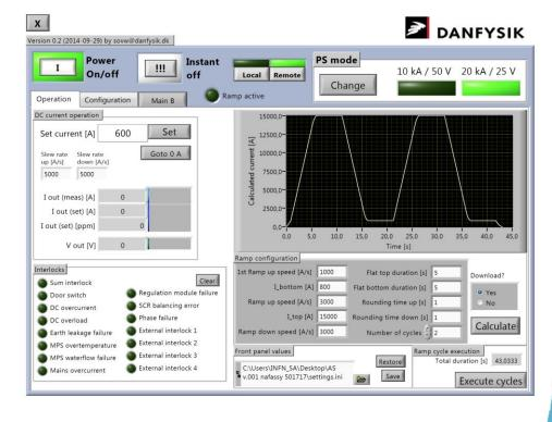
The output of a ramp control test, up to 15 kA, rate 3kA/s, flat top 5 s: white set profile, red measured profile.
