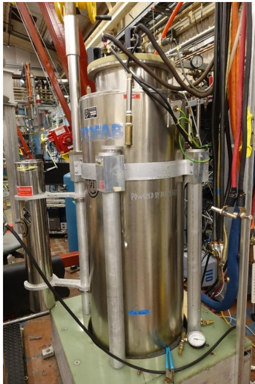
15 T solenoid SC magnet
