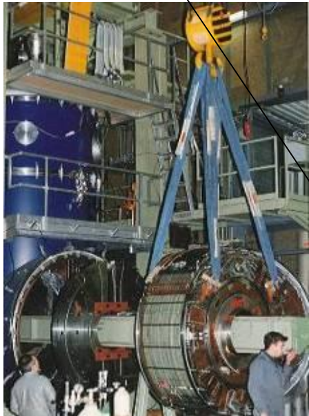
Possibility of coil testing in the main bore (Ø600 mm)
