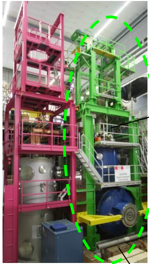
Vertical test well 94x144 mm 2 (separated vacuum)
