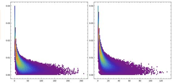
Figure 5.36: Electron scattering angle (mrad) versus the electron energy (GeV) for signal candidates, (a) in a model with  $m_A=800~{\rm MeV/c^2}$  and  $m_\chi=200~{\rm MeV/c^2}$  and (b) with  $m_A=405~{\rm MeV/c^2}$  and  $m_\chi=200~{\rm MeV/c^2}$ .
