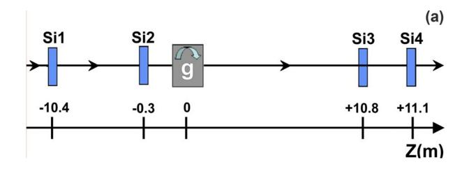
Particle angles were measured with the telescope of microstrip detectors with accuracy 3  $\mu$ rad
