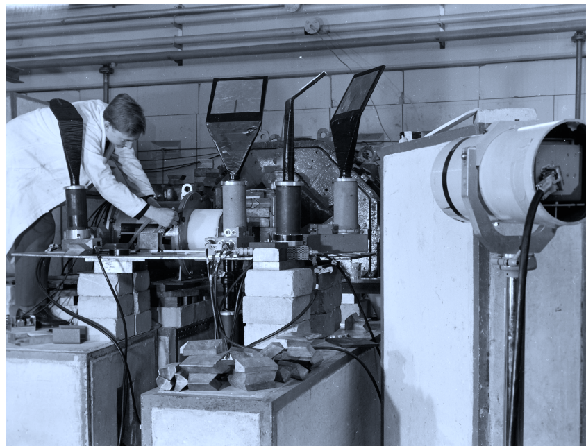
Fig. 9. The SC experiment to measure the \pi^+ \rightarrow \pi^0 e^+ \nu decay rate 37, 38 during installation.
