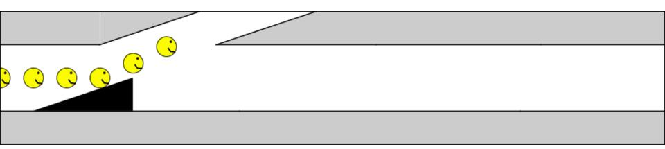
Asynchronous dump: kicker(s) fire when beam passes – kicked beam damage could tungsten collimators. TCDQ should protect
