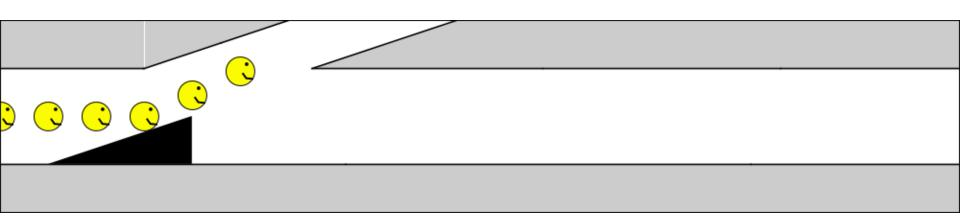
Asynchronous dump: kicker(s) fire when beam passes – kicked beam damage could tungsten collimators. TCDQ should protect
