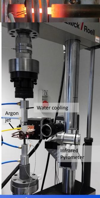
Quasi-static and medium strain-rate tests
