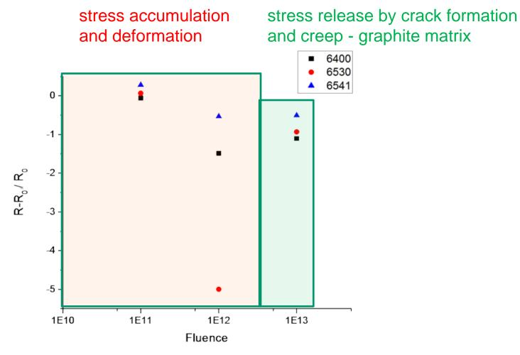
MG6541 (short fibers, Ti addition) smallest deformation
