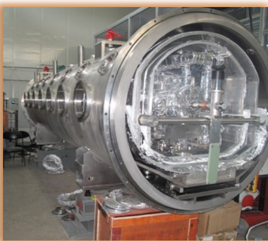
Assembly of a 5 MeV Spoke Cryomodule in IHEP Beijing (China)
