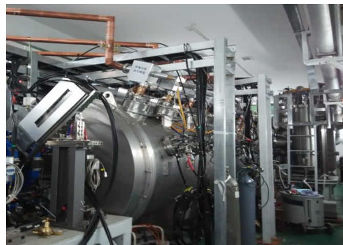
Assembly of a 5 MeV Spoke Cryomodule in IHEP Beijing (China)
