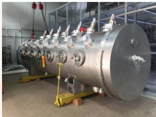
Assembly of a 5 MeV Spoke Cryomodule in IHEP Beijing (China)
