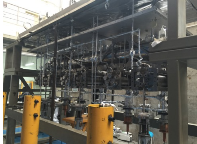
Assembly of a 5 MeV HWR Cryomodule in IMP Lanzhou (China)
