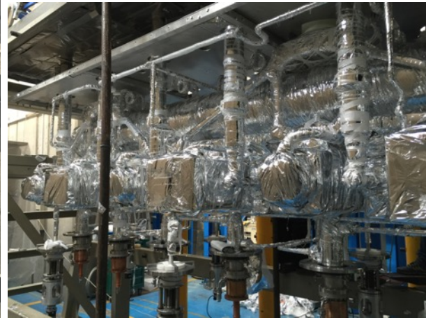
Assembly of a 5 MeV HWR Cryomodule in IMP Lanzhou (China)
