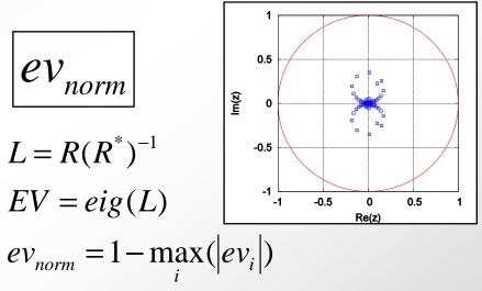
ev<sub>norm</sub> ... eigenvalue norm L ... matrix that determines the poles of the control loop
